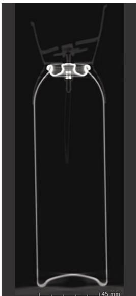
Figure 5: Right slice of oxygen boost can
